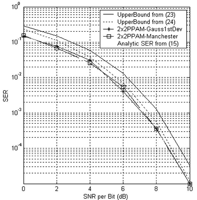
Fig. 4. Performance of a 4-ary BPPM UWB system with Gaussian first derivative pulses and Manchester pulses.
