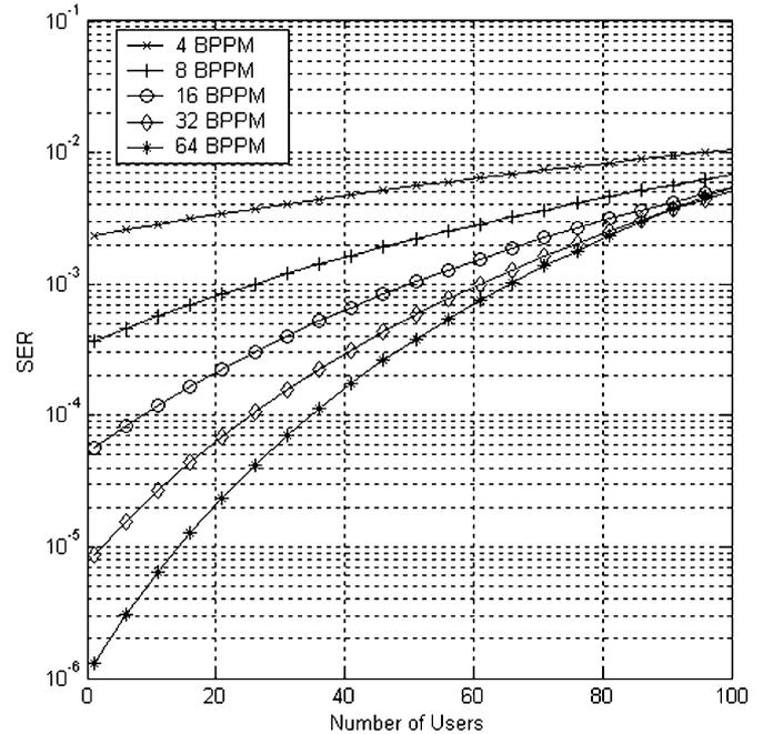
Fig. 8. Capacity of an  $N$ -ary BPPM UWB system with  $\rho = 500$ , SNR/bit = 7 dB and Gaussian first derivative pulses.
