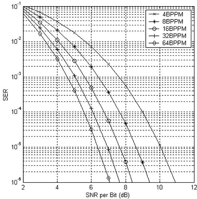
Fig. 6. Upper bound on error probability (24) for an  $N$ -ary BPPM UWB system.
