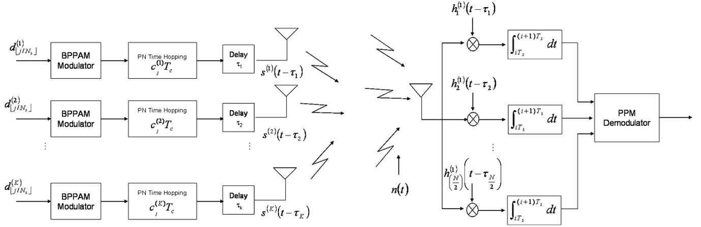
Fig. 1. System model of a time-hopping multiple-access  $N$ -ary biorthogonal PPM UWB system.
