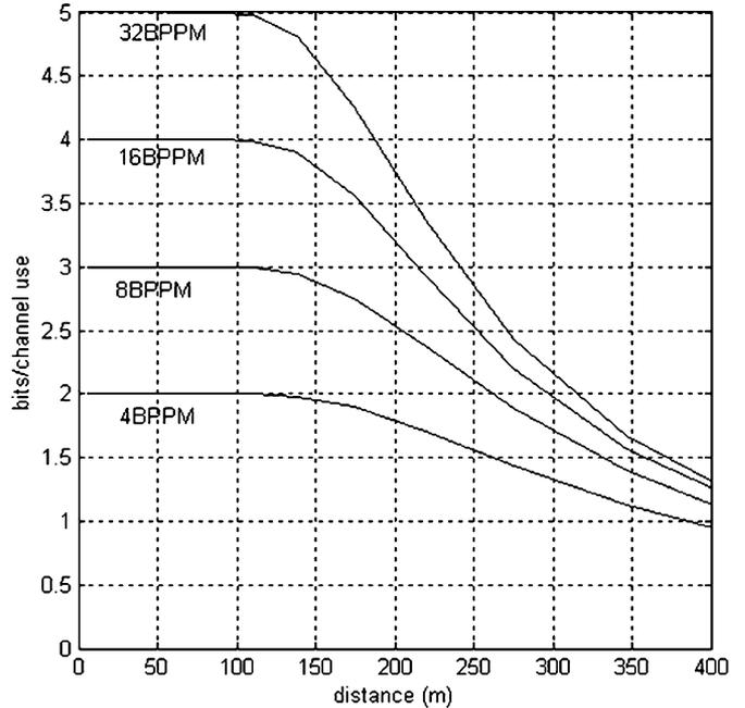
Fig. 3. UWB spectral efficiency as a function of range for  $n = 2$ ,  $G = 100$  and  $N$ -ary BPPM.
