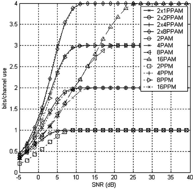
Fig. 2. Channel capacity with  $N$ -ary BPPM over an AWGN channel.
