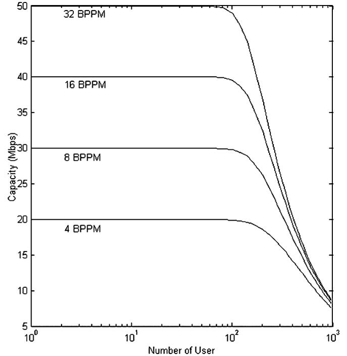
Fig. 7. Capacity of an  $N$ -ary BPPM UWB system with  $\rho = 100$ , SNR = 15 dB, Manchester pulses and  $T_p = 1$  ns.
