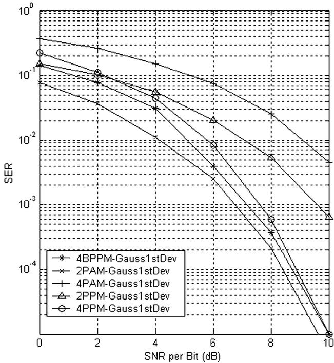
Fig. 5. Performance comparison between PAM, PPM, and BPPM with Gaussian first derivative pulses.
